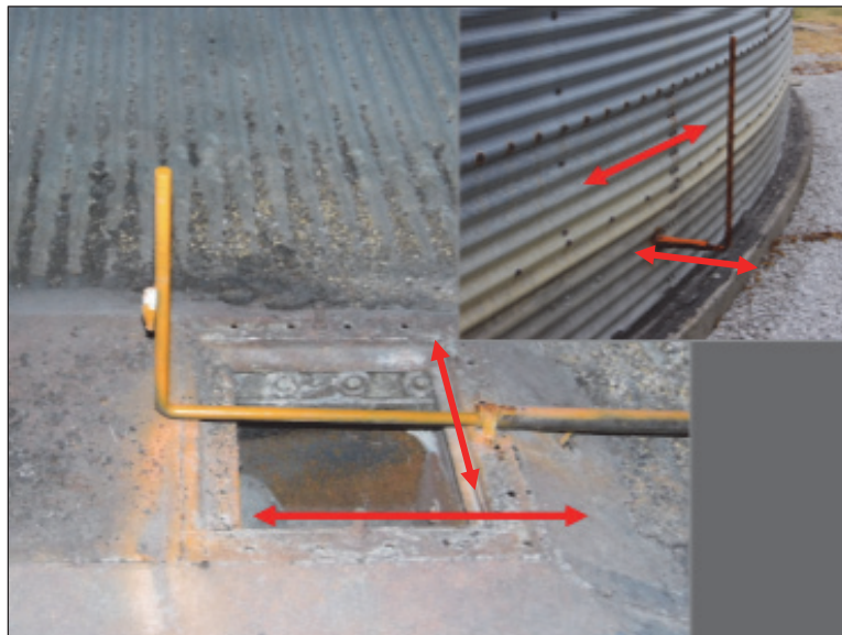
Figure 4. Rod over sump. An individual can move rod back, forth, and sideways to break up grain clumps.
