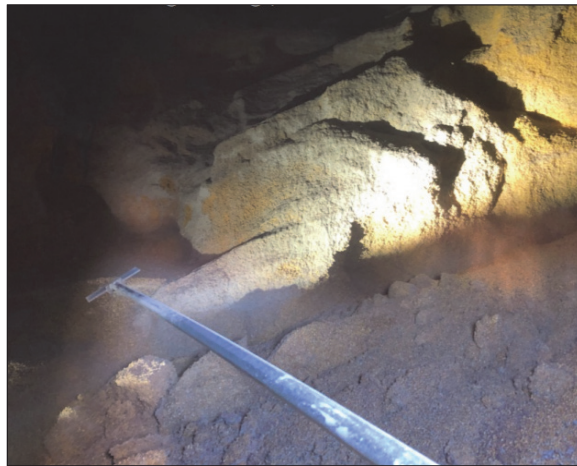
Figure 6. Extendable pole in action. Pole is used to break grain clumps blocking sump.
