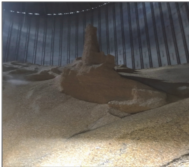
Figure 2. Example of grain tower (approx. 70 feet tall) composed of out-of-condition grain. (Lee, 2021).
